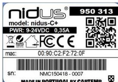
Figure 52 - Example: MAC: 00:90:C2:F2:72:0F is the hardware unique identifier
