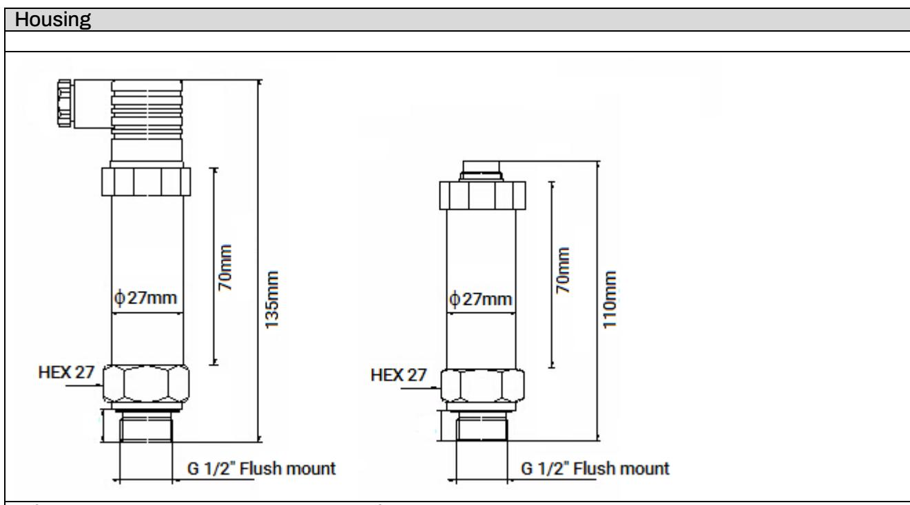
Left: device assembled with connector ISO 4400, flush mount diaphragm.
