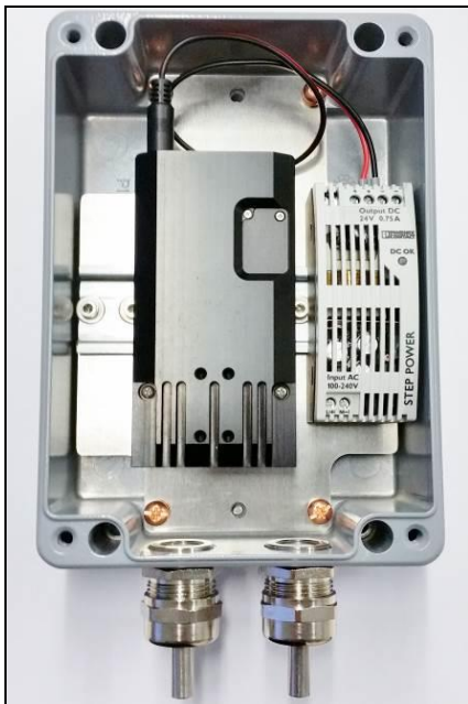
Figure 4: Protective housing with power supply [Part-No.: ACPINBPHPS]
